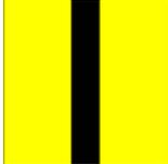
A yellow square signal with a thin white border and a vertical black bar in the center, representing a yellow light with two flashes.     |
